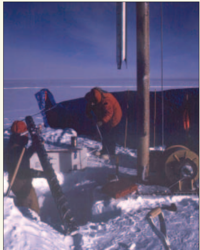
Fig. 3. Two drillers preparing to cut a new section of core in Antarctica. The person on the left is getting ready to attach the inner, rotating part of the drill to the outer, nonrotating shell, which is hanging from the drill cable. The driller on the right is using a tape measure to determine the depth of the hole. (Photo courtesy of Cara M. Sucher)
